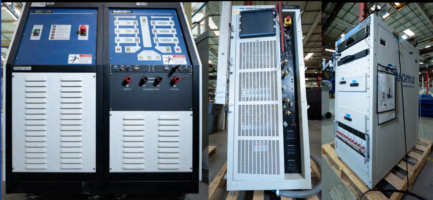
Battery Test Equipment
